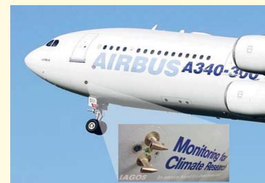
Fully automatic instruments are permanently installed on AIRBUS A330 and A340 aircraft operated by different airlines. The instruments are designed according to aeronautic standards and are approved by the European Aviation Safety Agency. Data are collected on each flight between take-off and landing (~500 flights per aircraft and year).
