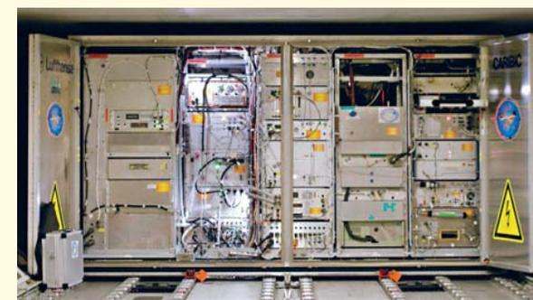
Each month, a cargo container with 19 instruments for measurements of atmospheric trace gases and aerosol is loaded on an AIRBUS A340 of Lufthansa, which is fitted with special provisions for sampling of gases and aerosol. After four flights, the container is brought back to the laboratory for calibration of the instruments and analysis of the samples collected during flight.
