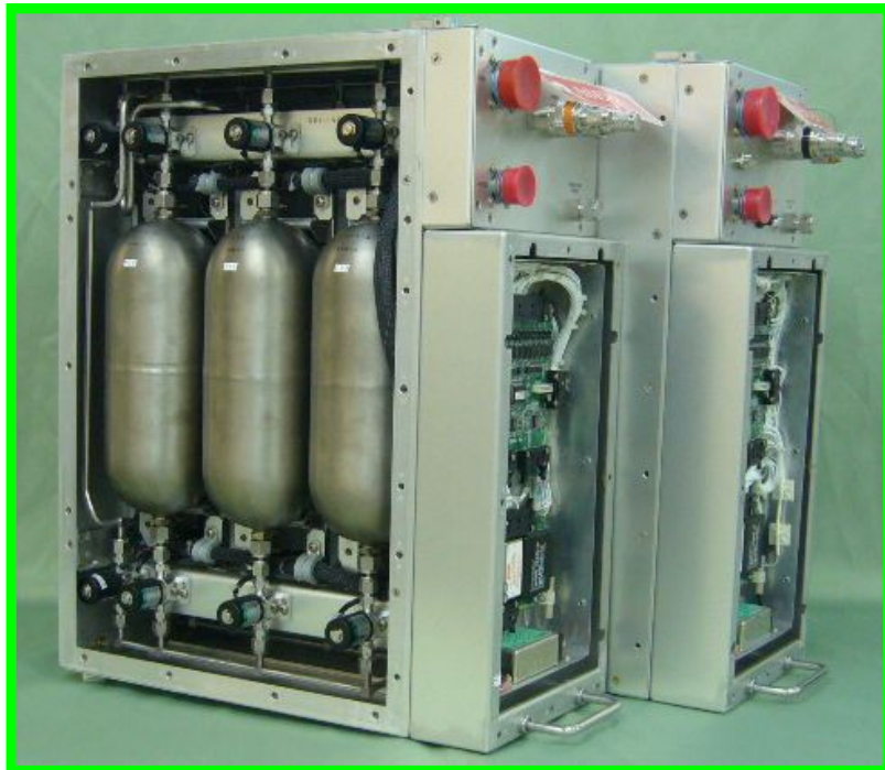
Automatic air Sampling Equipment
