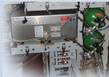
Figure 2.1: The pump of the analyzer supplies the instrument with sample air, which enters the system through the inlet. The air is then measured in situ by the temperature and pressure controlled analyzer. In-flight calibrations guarantee the quality of the measurements. The sample flow leaves the instrument to the atmosphere through the exhaust line, connected through the flange that carries the inlet
