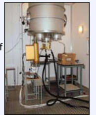
MICC – showing CAS and CDP cloud instruments
