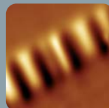
MFM - AFM Image of Calibration Grating at 4.2K
