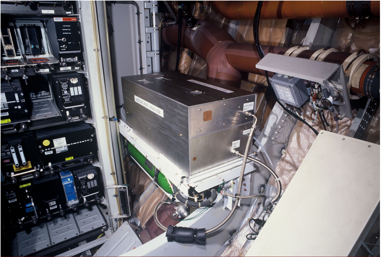
The MOZAIC NO y instrument in the avionics bay of a Lufthansa A340-300
