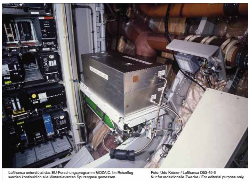
Figure 4. MOZAIC instrument for autonomous \text{NO}_y measurements in the avionics compartment of an Airbus A340. The new IAGOS equipment will be installed in the same location. (Photo by Udo Kröner, Lufthansa).
